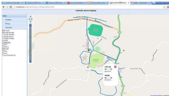
Figure 6: OSM layer with water pipelines with details
